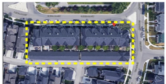
Example: Density of 42.2 Units per hectare - 12 Townhouse Units with rear lane garages - Site Area: 0.3 ha
