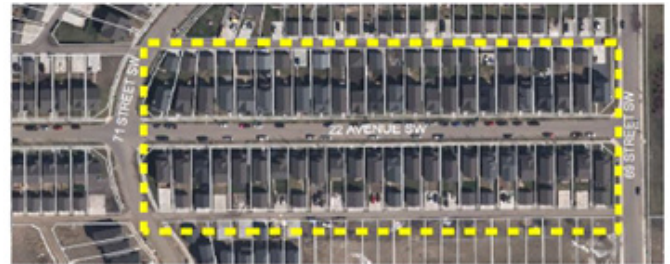
Example: Density of 30 Units per hectare - 48 Single Detached Homes with rear lane garages - Site Area: 1.60 ha
