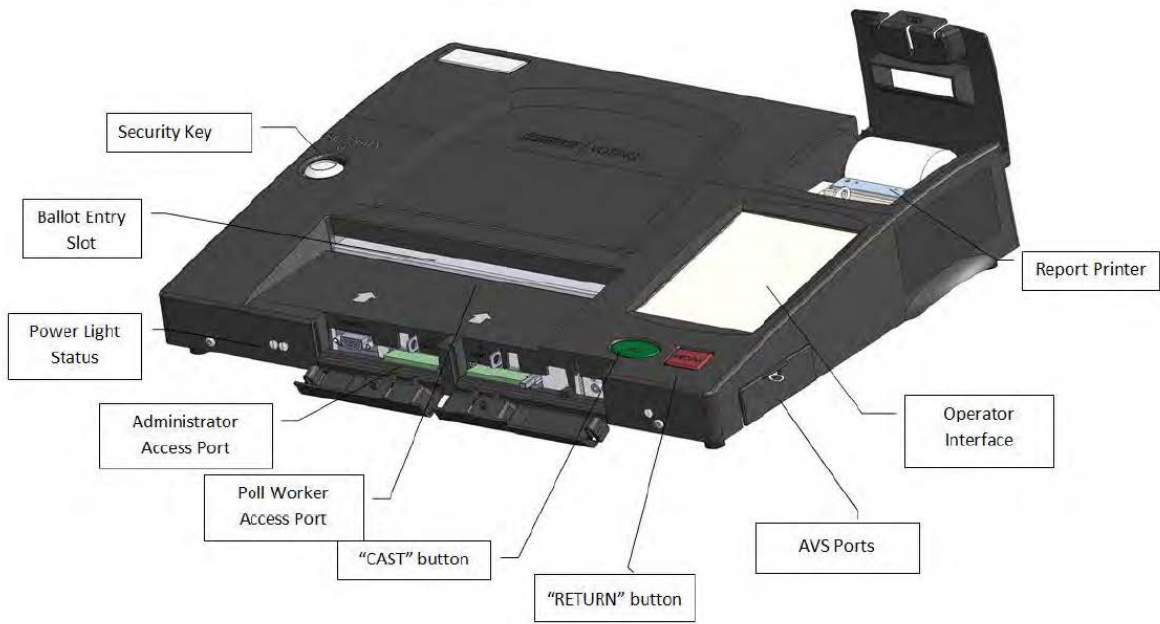
Figure 1: Front View of ImageCast® Precinct Tabulator
