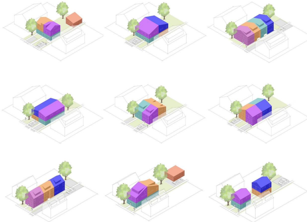
Examples of how four units can be accommodated on a lot (Source: Province of British Columbia)
