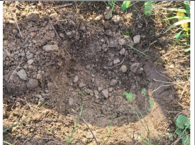
IMAGE 6 TEST PIT IN PROGRESS: DISTURBED
