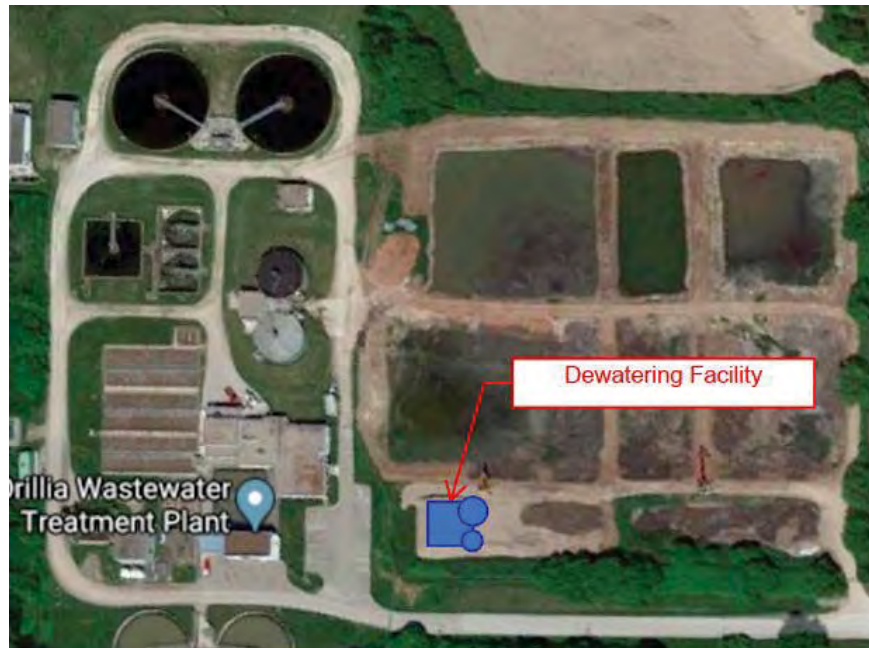
Figure 23 – Proposed Location of the Dewatering Facility
