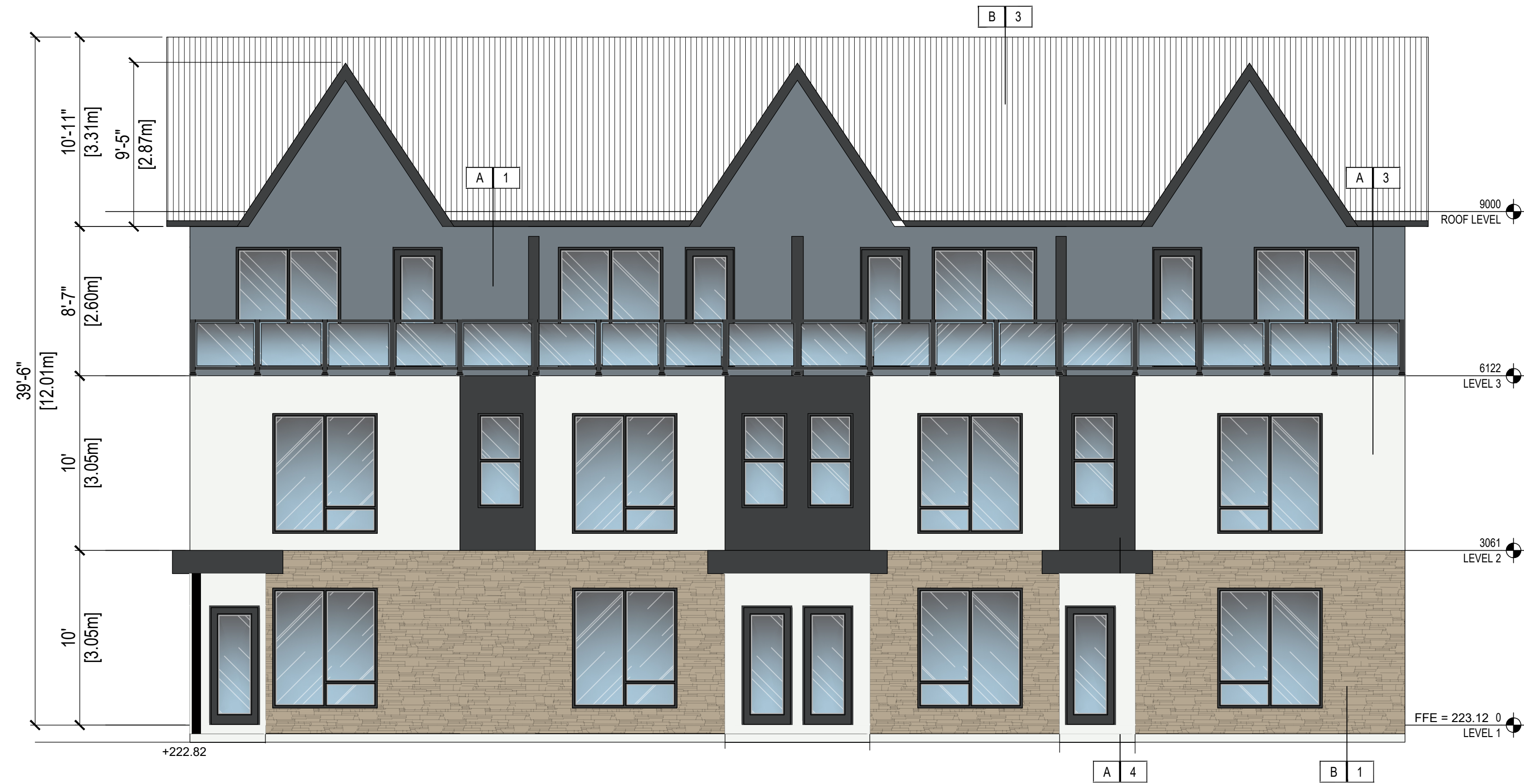
1 NORTH ELEVATIONS 3/16" : 1'-0" (INTERIOR SIDE YARD PARKING)
