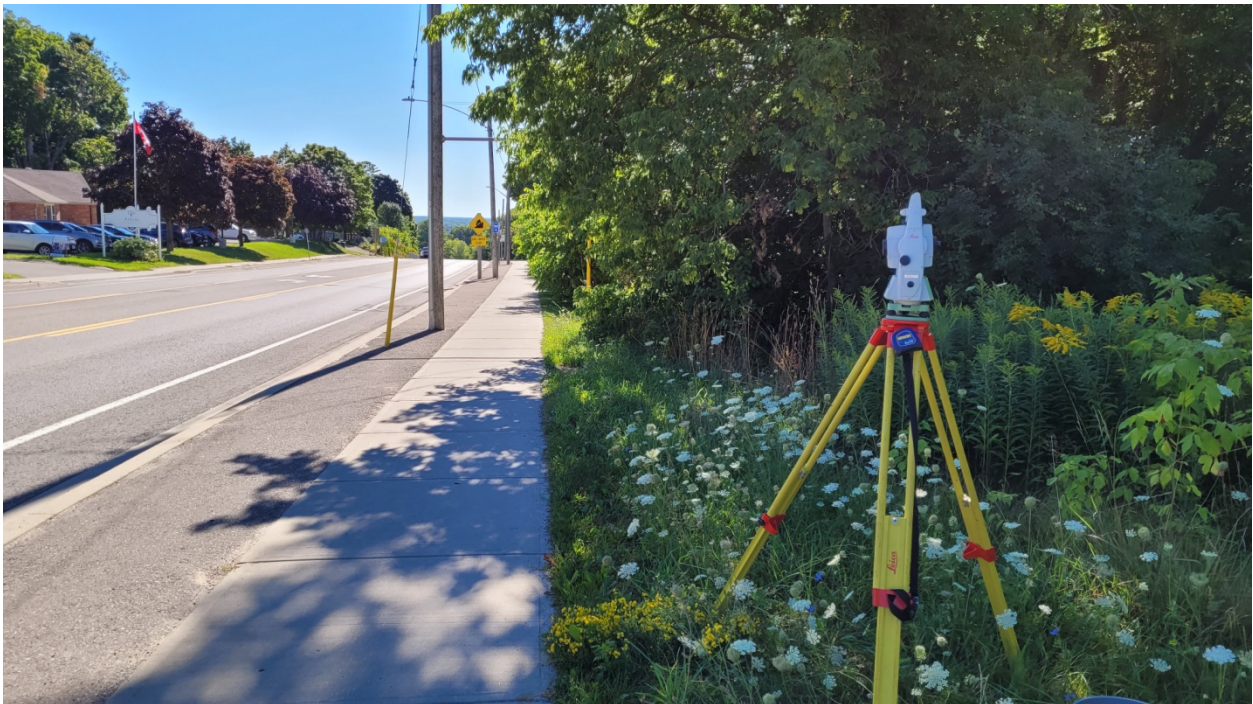
Figure 2 - Apparatus for Sight Distance Analysis
